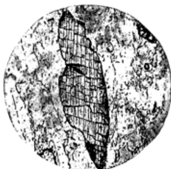
2. Kyanite. Showing cleavages and high refractive index.
